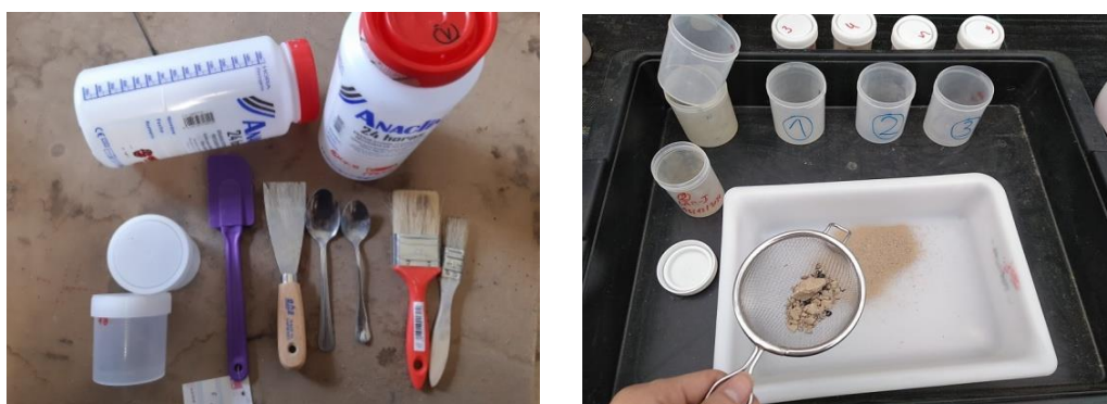
Figure 5 Detail of the material used in the process of soil collection in the Gerlach box of the experimental field of cover crop versus tillage carried out in Elvillar (Araba) from 1/04/20 to 31/03/2022.
