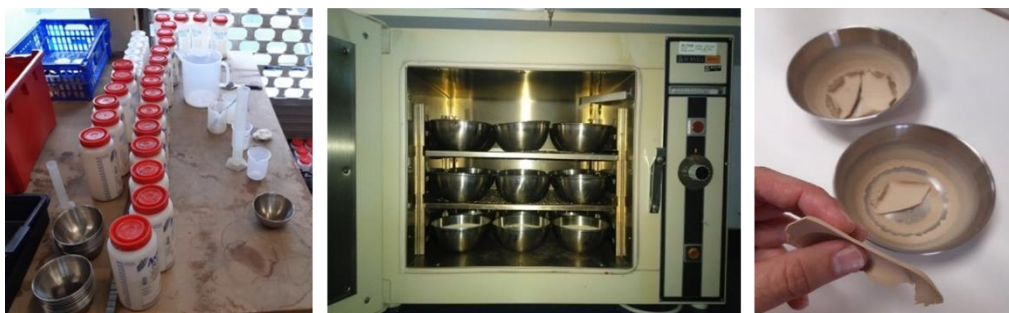
Figure 6 Water samples processing and measurement of soluble solids in the canister of the cover crop versus tillage experimental field carried out in Elvillar (Araba) from 1/04/20 to 31/03/2022).
