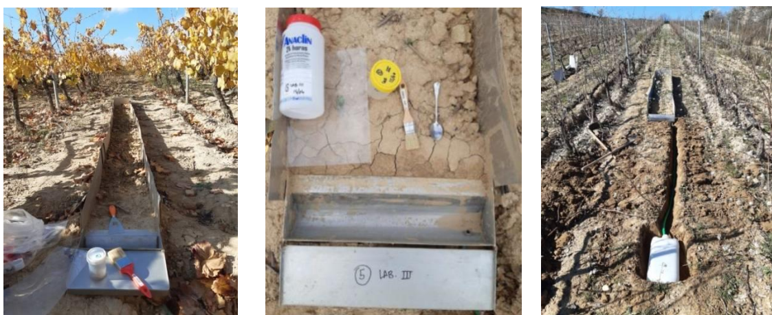
Figure 4 Installation of the experimental micro-plots for measuring erosion, with Gerlach boxes and water storage drums for the trial of vegetation cover versus ploughing carried out in Elvillar (Araba) from 01/04/2020 to 31/03/2022.
